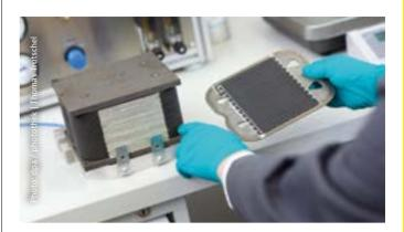
The dismantling of fuel cell stacks — the heart of fuel cell power systems — at the end of their use lives requires a high level of manual labor, but that may not be the case for long. The Open Hybrid Labfactory in Wolfsburg is working on the world's first pilot line for fully automated stack dismantling.
